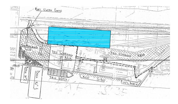
The blue zone indicates the location of the ICD, and the lake container terminal is indicated as TEU working area. The two zones are separated by an existing roadway, and this point may need further study in the future. The dotted line shows the proposed split of land between TRC (north of this line) and Marine Services Co (south of the line)
